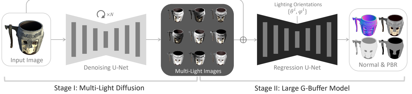
Figure 2. Framework Overview. Multi-light diffusion generates multi-light images from an input image. These images with corresponding lighting orientations are then used to predict surface normals and PBR materials with a regression U-Net.
